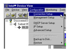
Figure 19. Configuring a VPN Tunnel. Select Connection Setup from the Configuration menu.
